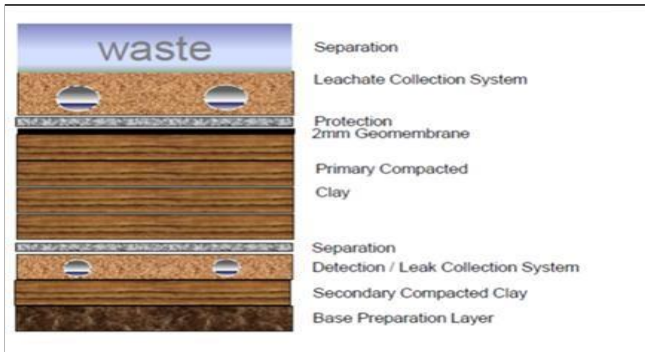
Figure 1.1: The different lining layers of the construction of the pollution control dam
